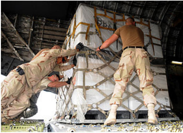
Figure 7. Depiction of a 463L pallet with multipack containers in Al Taqqadum, Iraq (Jan. 9, 2009). Seabees assigned to Naval Mobile Construction Battalion (NMCB) 7 and airmen of the Air Force Expeditionary Logistics Readiness Squadron Detachment 4 maneuver 463L pallets into an Air Force C-17 for transportation. 50
